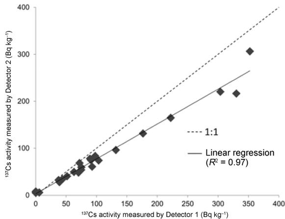
**Figure 5.** The comparison between the  $^{137}\text{Cs}$  measurements of a subset of samples ( $n = 16$ ) performed with two different HPGe detectors; detector 1 is housed by the Physics Department at the University of Basel (CH) and detector 2 is housed by the State Laboratory Basel-City (CH).
